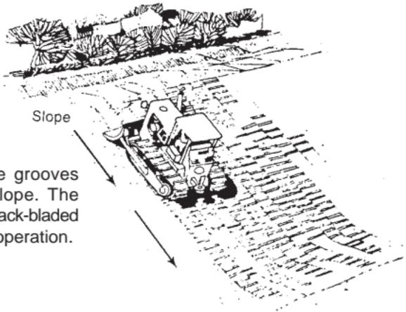
Bulldozer treads create grooves perpendicular to the slope. The slope face should not be back-bladed during the final grading operation.
