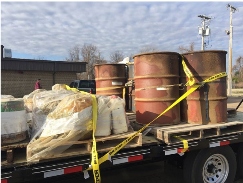
Figure 3. Secure the load with ratchet straps.
