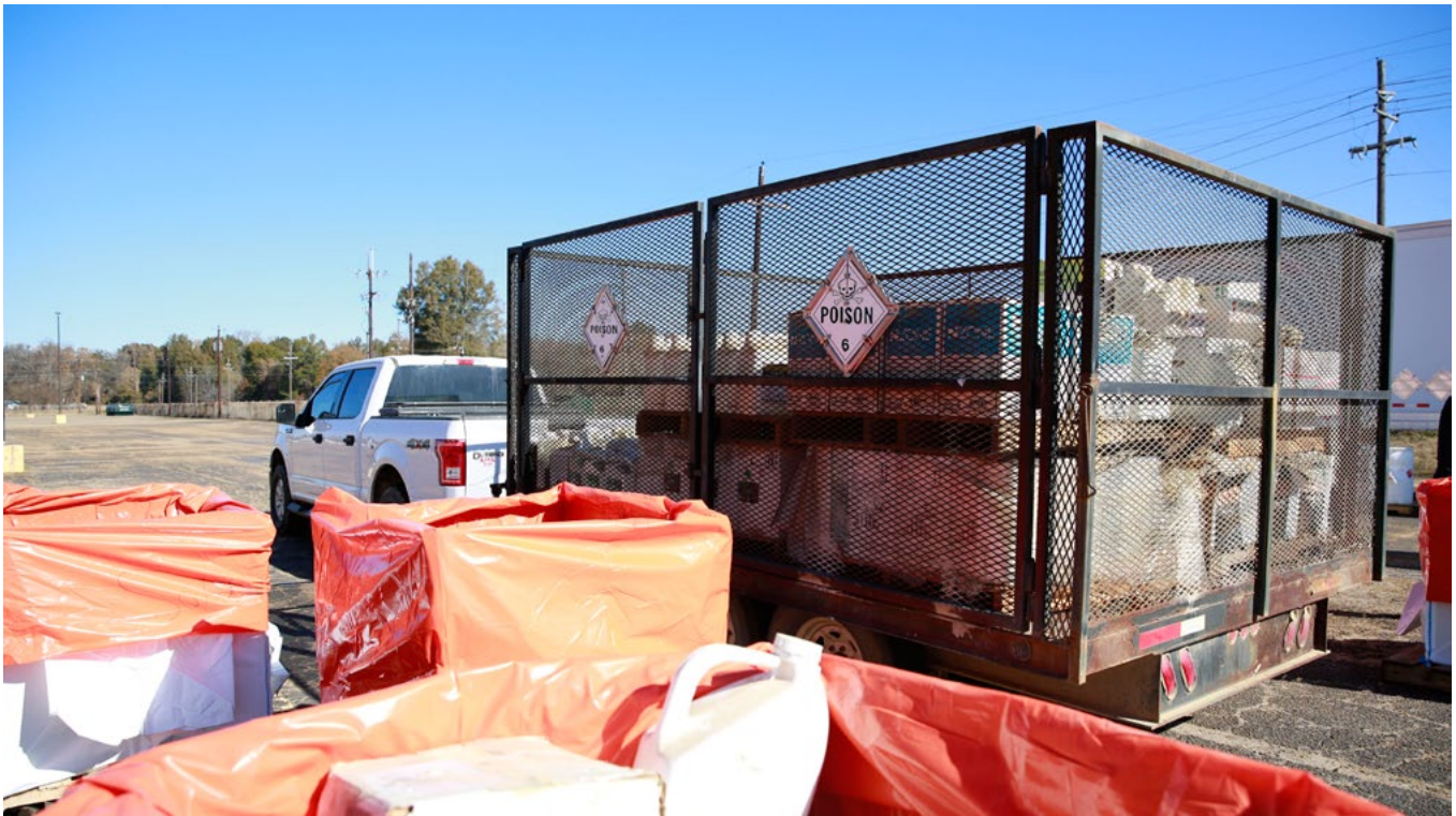
Figure 1. Loads over 1,000 pounds must display placards like the one shown here.
