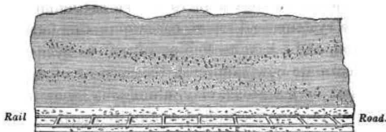
The cut is about fourteen feet through a red clay, which, all along for more than half a mile, contains a most remarkable stratum of pebbles. The pebbles begin to appear about four feet from the surface, and continue for about ten feet downwards, in different layers, as it appears in the diagram. They are so close and thickly crowded that it must have been impossible to dig the
