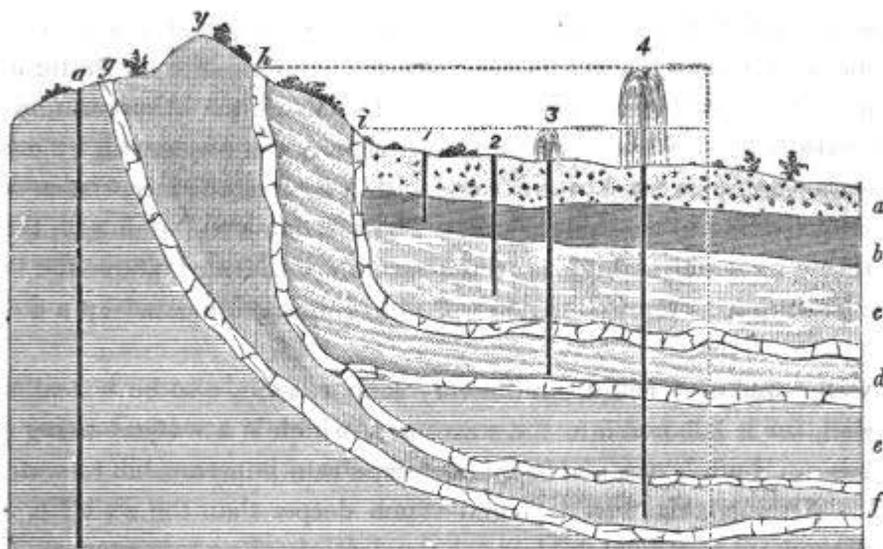
Let the strata *a, b, c, d, e, f*, be all water-bearing strata—that is, strata which are composed of loose material, such as sand, gravel, pebbles, etc. A well bored at 1 will not be a real artesian well, whose water rises above the surface, for two reasons :
