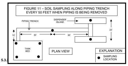
If any of the sidewalls of the piping trench excavation appear to be contaminated, the sidewalls must be sampled. Samples must be collected from the areas of the sidewalls that appear to be the most contaminated. However, sampling must be conducted so that no more than 50 feet exists between any two sampling points.
