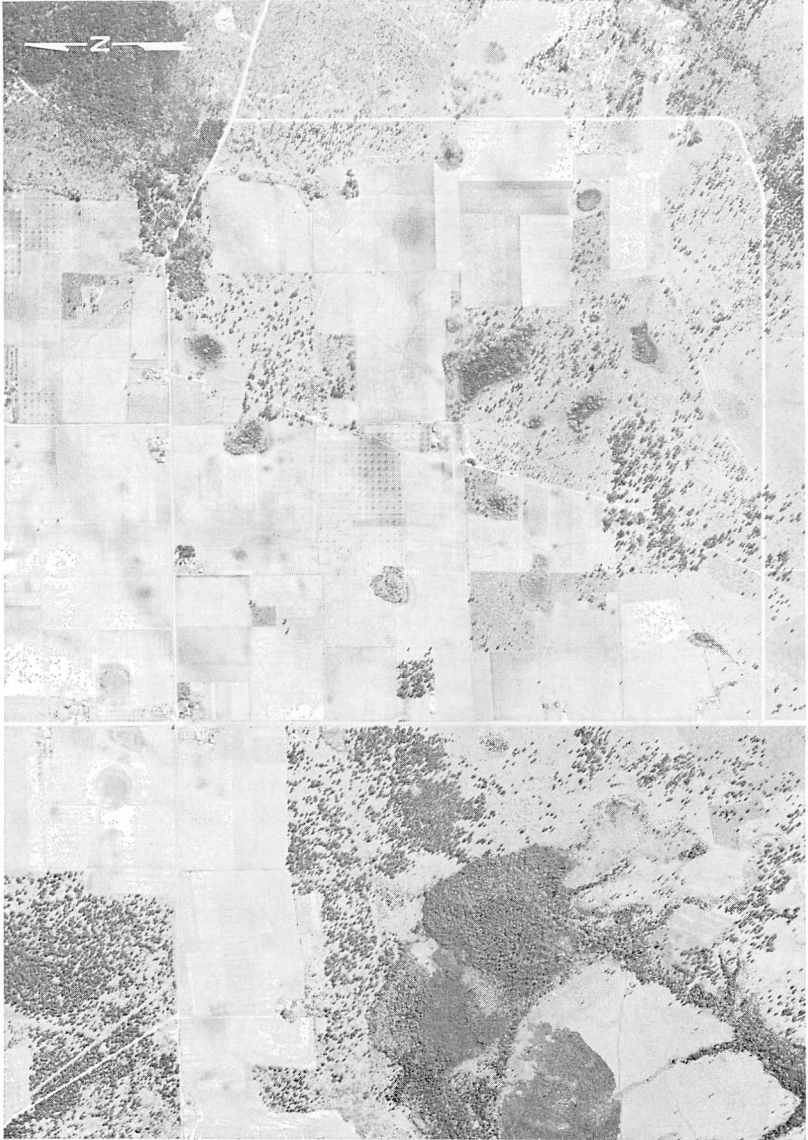
Figure 8.—Aerial photograph of Citronelle or High Terrace terrain showing circular depressions. At least 12 depressions are shown. The road intersection to the northwest marks the common corner of secs. 20, 21, 28 and 29, T. 3 S., R. 6 W. Section 28 is bordered by section-line roads. March, 1942.
