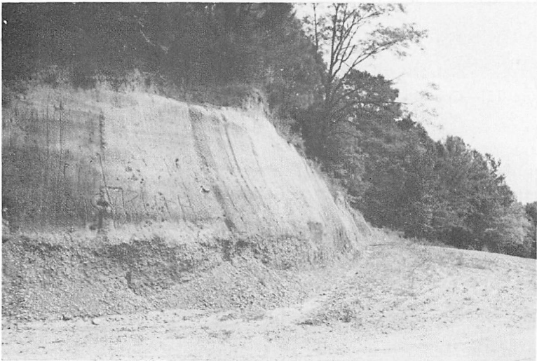
Figure 16.—Sharply defined contact of terrace gravels and loess at intersection of county roads near center of SW.¼, Sec.32, T.13N., R.4E. June 14, 1966.
