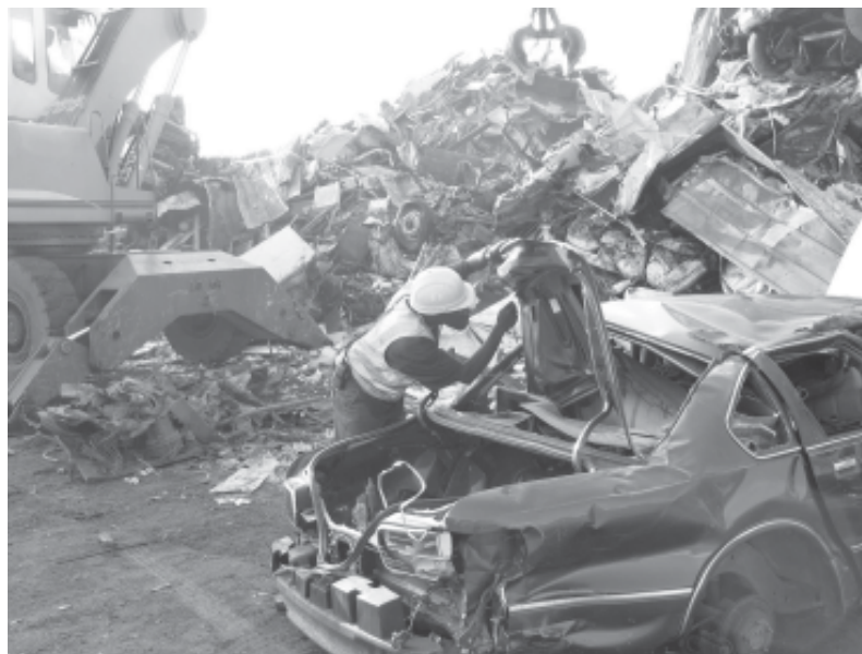
Vehicle Mercury Switch Recovery
