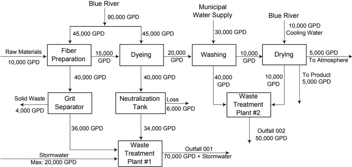
Schematic of Water Flow
