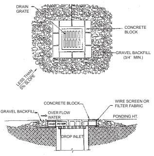
Source: Florida Erosion and Sediment Control Inspector's Manual
