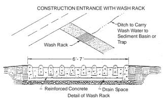
Source: Mississippi's Planning and Design Manual for Control of Erosion, Sediment and Stormwater.
