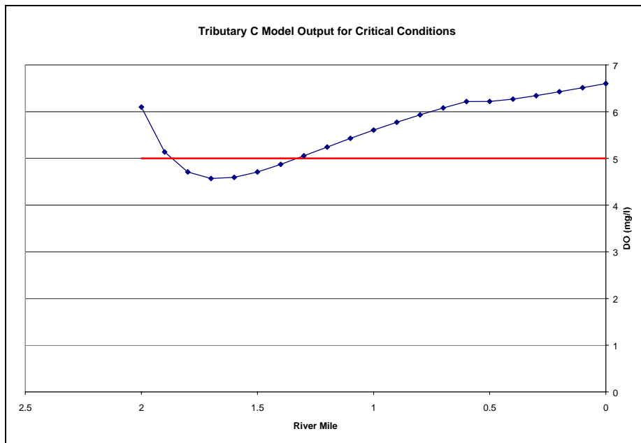
Figure 23. Critical Condition Model Output for DO in Tributary C
